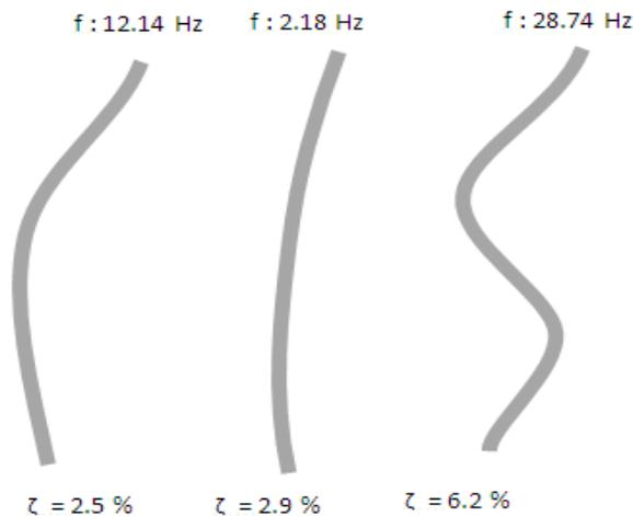
Figure 1. The first three longitudinal modes together with natural frequencies and damping ratio
